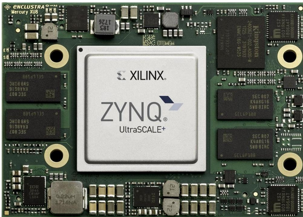
*The Enclustra Mercury+ XU8 is based on the Xilinx Zynq UltraScale+ MPSoC and is optimized for applications that need to process large amounts of data in the shortest possible time. (Picture: Enclustra GmbH)*
