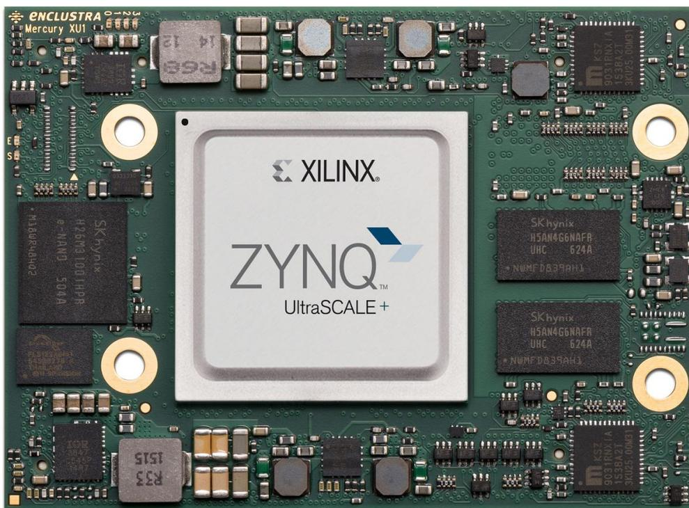
*The Enclustra Mercury+ XU1 is supremely equipped to handle even the heaviest of resource-hogging applications, despite having a footprint of just 74 × 54. (Picture: Enclustra GmbH)*
