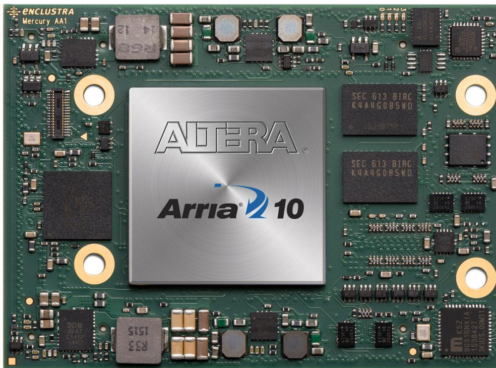
The Mercury + AA1 is the first module from Enclustra based on the Intel Arria 10. (Picture: Enclustra GmbH)
