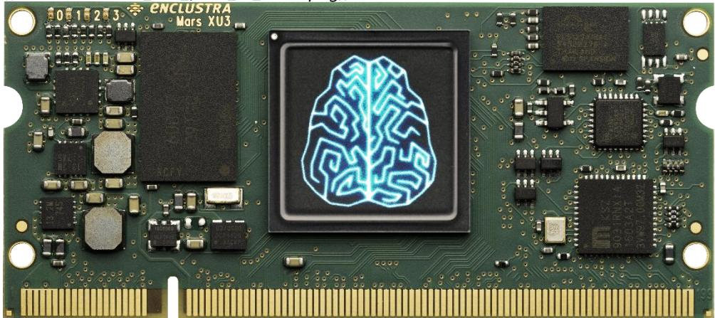
The Enclustra Mars XU3 System on Module (SOM) is the smallest Xilinx Zynq UltraScale+ MPSoC-based module from Enclustra. (Picture: Enclustra GmbH)
