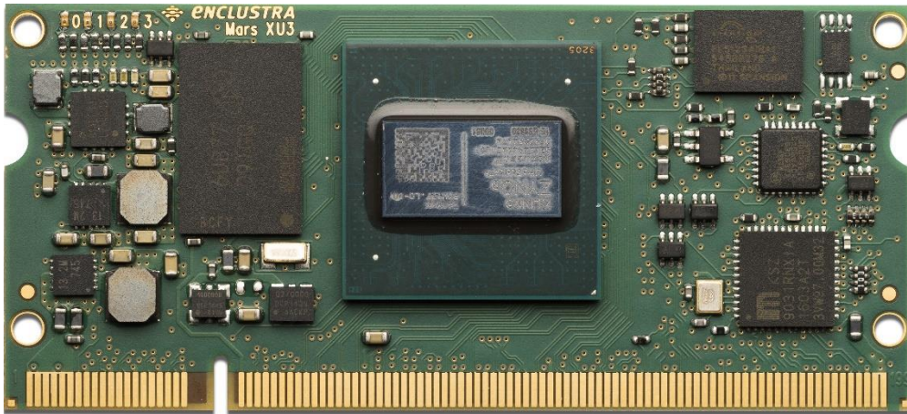
The Mars XU3 is the smallest Xilinx Zynq UltraScale+ MPSoC-based module from Enclustra. (Picture: Enclustra GmbH)
