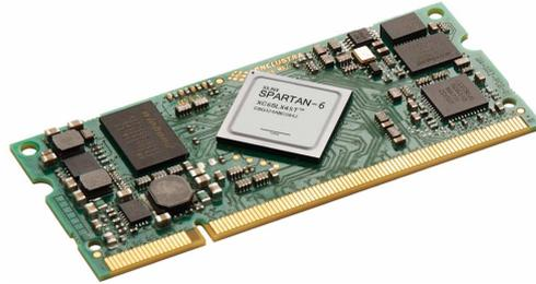
The Mars MX1 module in particular is a perfect platform for implementing drive control systems. Beside its optimization for low cost and SOPC systems, it also contains two ethernet physicals to support real time Ethernet standards such as EtherCAT.
